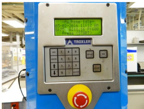
Gyratory compactor screen display showing system is idle
